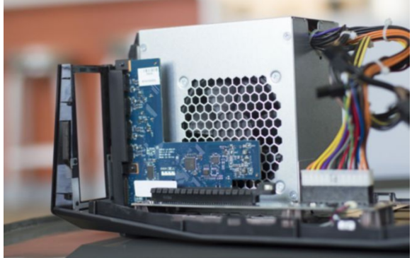
A single x16 physical PCIe Gen 3 slot sits empty in the Amplifier.
