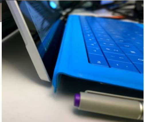
A Surface Pro 3 keyboard connected to a Surface 3 works, but the two won't create the secondary magnetic connection to tilt the keyboard.
